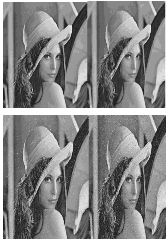
Fig. 1. Salt & Pepper noise (15%). Top row: original image, noise image; middle row: results of AWFM2 and DS-FIRE filter; bottom row: results of IFC and median filter
