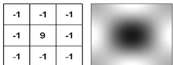
Figure. 4 3x3 ‘High Boost’ kernel and its corresponding Fourier spectrum. Note that the sum of the kernel elements is one so the image intensity in homogeneous regions will be unchanged. The gray center of the Fourier spectrum indicates that low frequencies are only partially attenuated so tonal detail is retained
