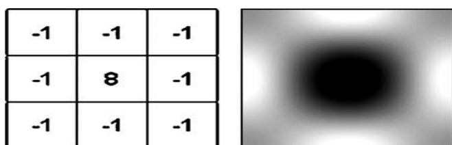
Figure. 2 A Laplacian kernel calculates the second derivative of the image intensity. The 3 X 3 Laplacian kernel and its Fourier spectrum are shown here. Note that the sum of the kernel elements is zero, so the output is not scaled. The Fourier spectrum confirms that convolution with this kernel acts as a high pass filter
