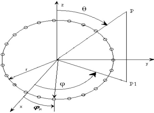
Figure.1. Uniform Circular Array of N isotropic elements
