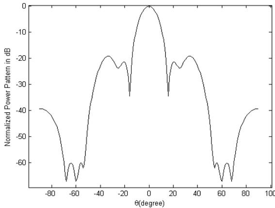
Fig.3. Normalized power pattern with wide null
