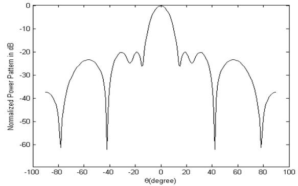
Figure.2. Normalized power pattern with multiple nulls
