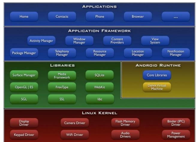
Figure. 1 Android Architecture (developer.android.com, 2011)
