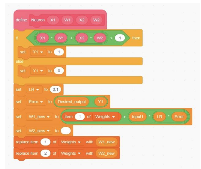
Figure 14. Work Sample. Unfinished task to calculate weight recovery (source: MIT Scratch Tool)
