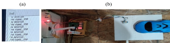
Figure 6.31 (a) Results on shell showing no violation (b) overall view of the System setup when red led glows and there is no violation.
