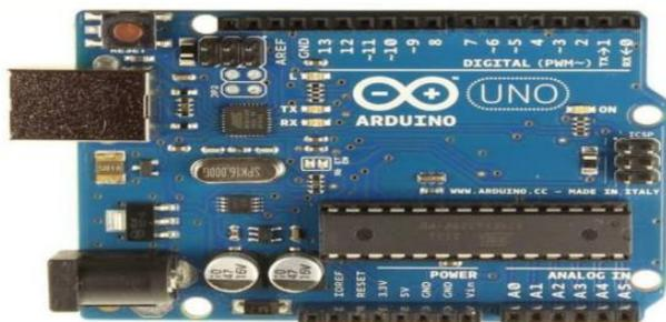
Fig 4: Arduino uno micro-controller
