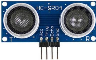
Fig 2: HC-SR04 Ultrasonic sensor
