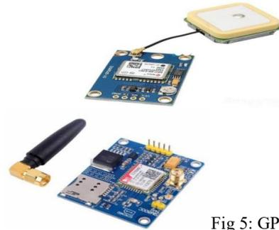
Fig 5: GPS and GSM module
