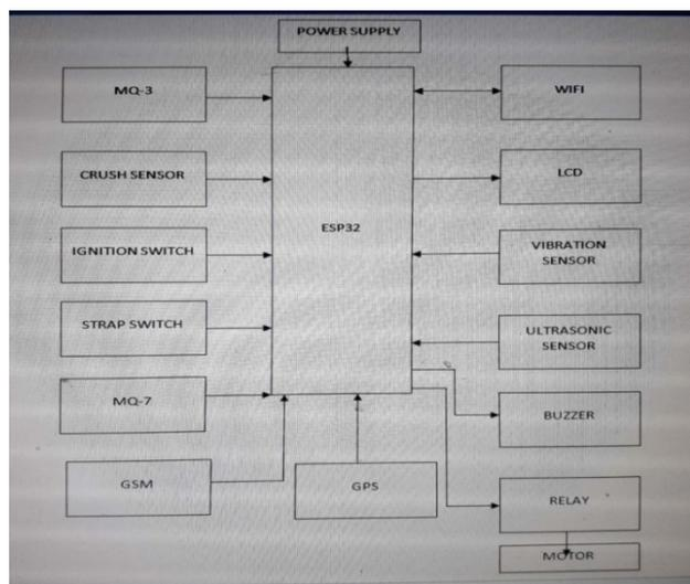
Fig. 1. Block diagram of smart helmet to detect the hazardous situations and accident alerts
