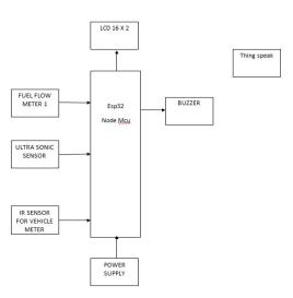
Figure 3:Block Diagram of Fuel Monitoring System
