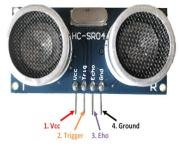
Figure 7: Ultrasonic Sensor
