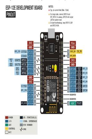
Figure 8.ESP-12E Development Board
