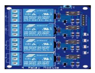
Figure 5. Opto-Isolated 5v Relay Module
