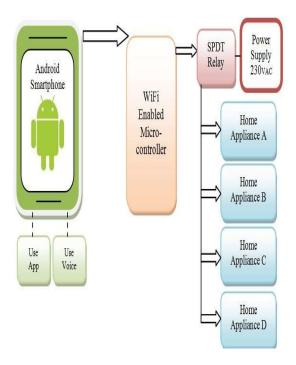
Figure 2. Smart Switch Board WorkFlow
