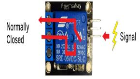
Figure 7. Normally open vs Normally closed
