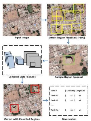
Figure 2. Overhead water tank detection from Satellite image using Faster
