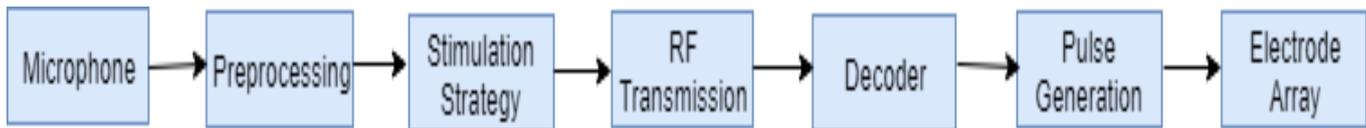
Fig: 1: A diagram representing the complete CI system.
