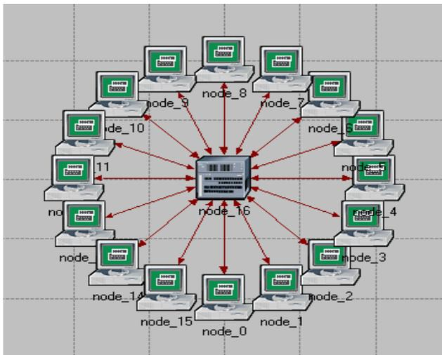
Figure. 1: Fast Ethernet Network for 16 Ethernet Stations
