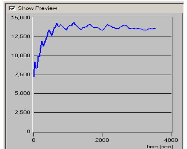
Figure. 7: Throughput (bits/sec) of 16 users for FDDI
