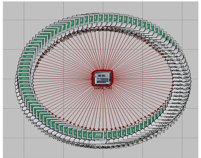
Figure. 2: Fast Ethernet Network Model for 100 Ethernet Stations
