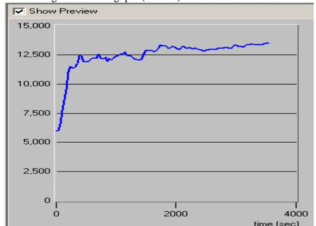
Figure. 8: Throughput (bits/sec) of 100 users for FDDI
