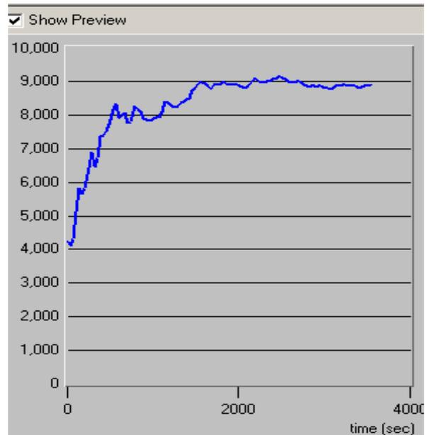
Figure. 6: Throughput (bits/sec) of 100 users for Fast Ethernet
