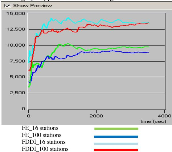
Figure. 9: Graph comparing throughput of Fast Ethernet and FDDI
