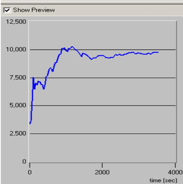
Figure. 5: Throughput (bits/sec) of 16 users for Fast Ethernet
