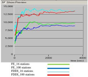
Figure. 9: Graph comparing throughput of Fast Ethernet and FDDI
