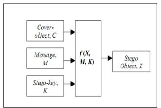
Figure 1: Basic Steganographic model [1].
