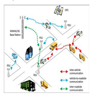
Figure-3. V2V communication architecture.
