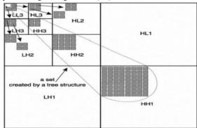
Fig.2: Wavelet sub-bands in STD-BCS-SPL.
