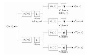
Figure 5: Image decomposition using Wavelet Transform.
