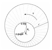
Figure 4: Normalization process
