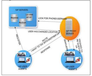
Figure 2. Flow of SIP connection between components
