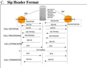
Figure 3. Illustration of an IP Phone call using SIP flow graph
