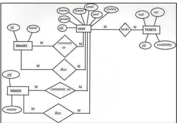
Figure 1. Entity relationship diagram. Table I. Schema design
