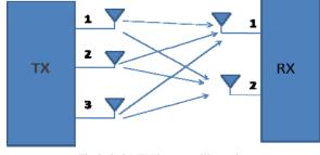
Fig 2: 3×2 MIMO system illustration
