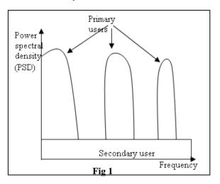
In Spectra Underlay, the level of the interference caused by the cognitive users to the primary users is governed by the cognitive radios. The cognitive users can transmit on the given band of the spectra only if the interference level is under the tolerable limit.
