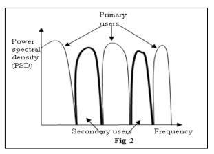
In spectra overlay, a CR user has information about message and/ or the encrypting strategy of other users. The noncognitive data transmission is assisted by this information and the interference with primary users is avoided by presubtraction. CR overhear the primary nodes communication and improves the communication. Spectra overlay provides better transmission with flexible control compared to spectra underlay. [7]
