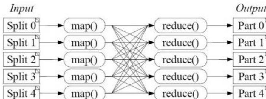
Fig 3. Map Reduce Block Diagram
