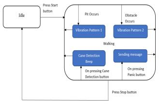
Fig 8. State Diagram of Smart Cane
