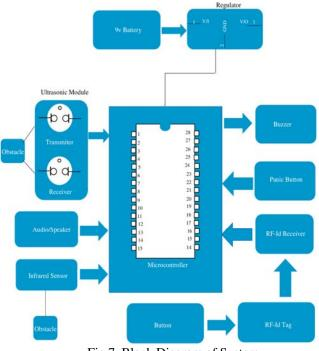
Fig 7. Block Diagram of System
