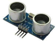
Fig. 1. Ultrasonic Sensor - HC-SR04
