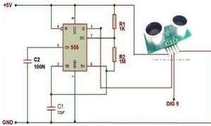
Fig. 4. Ultrasonic Sensor Circuit
