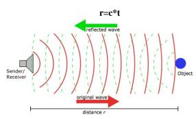
Fig. 2. Ultrasonic wave distance measure
