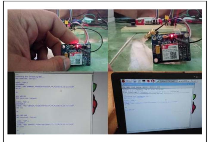
Figure 6. Module Notification SIM800L & AT Command
