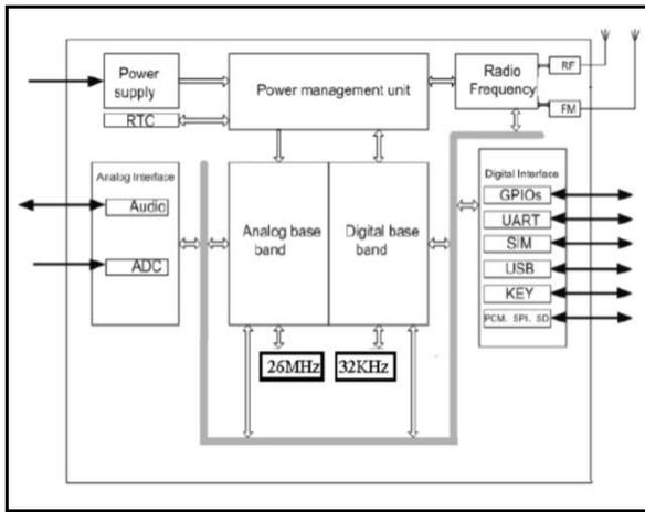
Figure 1. Sim8001 Diagram (Simcom)[9]
