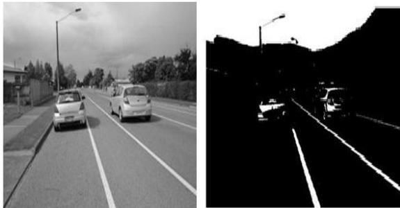
Fig 3: (a) Grayscale Image (b) Binary Image [16]
