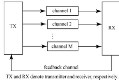
Fig.1. A Multichannel system with ARQ
