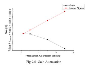
This graph shows the when gain increase attention also increase. Increasing attenuation coefficient from 0.2 to 5 db/ km.
