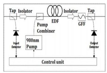
Figure 2: The EDFA setup with 980 nm pump vitality
