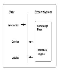
Figure 2. Structure of Expert System
