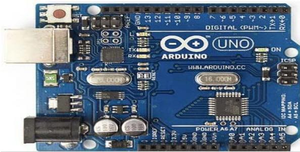
Figure 2. Arduino Uno Board
