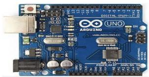
Figure 2. Arduino Uno Board
