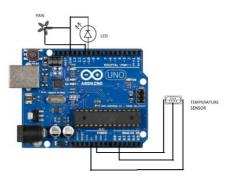
Figure 1. Schematic Diagram of Various Modules Figure 1 represents the connections of Arduino Uno with the LED,LM-35 and a DC motor.
