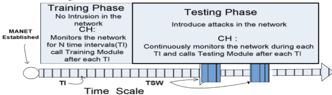
Figure 2: Time based operation of GIDP
