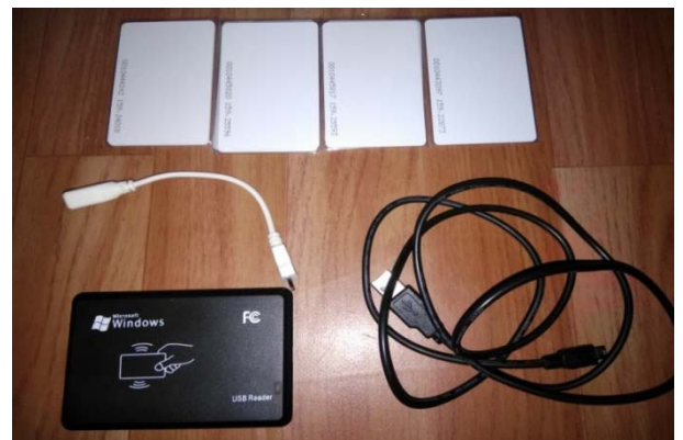
Fig 12: RFID Detector and RFID tag
