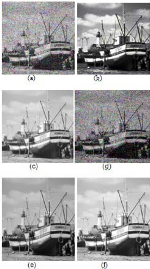
Figure 9.output host images obtained after applying (a) Gaussian filter attack (b) Speckle noise (c) Sharpening (d) Salt and pepper noise (e) without attack (f)Average filtering
