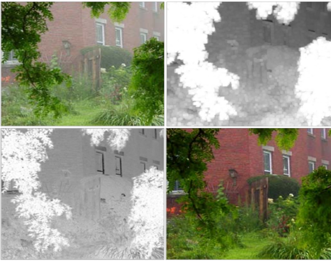
Figure 1. An overview of proposed dehazing approach. Top-left: original hazy image. Top-right: dark channel prior. Bottom-left: Transmission filtered map. Bottom-right: picture without haze.
