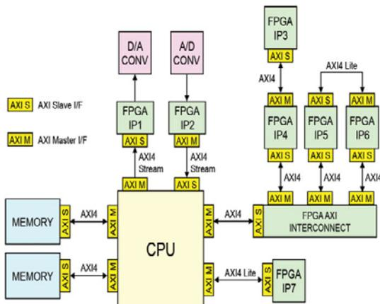
Fig 2: Architecture of CPU after connecting FPGA’s
