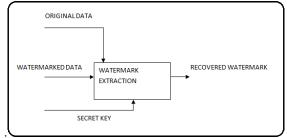
Fig 1: A Simple Diagram of Watermarking System.
