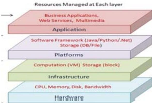
Fig 1: Intercloud Layered Architecture
