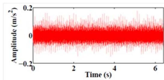
Figure 2: Comparison of time domain signals at 30 Hz and at load 100W of (a) Healthy gearbox; (b) Faulty gearbox
