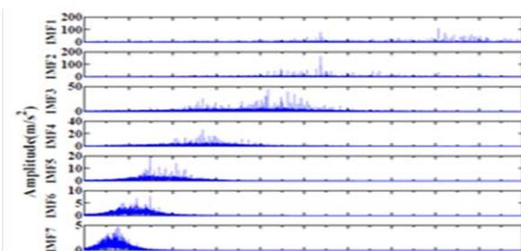
Figure 5: Fast Fourier Transform of the extracted IMF revealing gear mesh frequency
