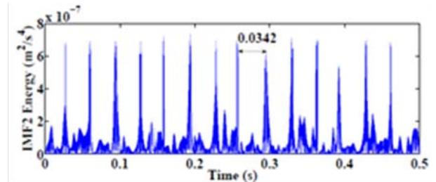
Figure 7: IE of IMF3 vibration signal of faulty gearbox
