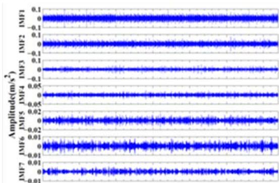
Figure 4: IMF of a faulty gearbox
