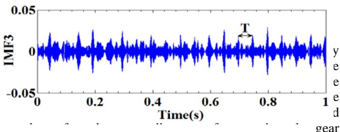
Figure 6: IMF3 vibration signal of a faulty gear
