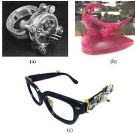
Fig. 6. Examples of wearable sensors using narrow-band communication technology. (a) Oxygen saturation and heart rate ring sensor . (b) e-AR sensor for detecting gait impairment . (c) Clip-free eyeglasses for measuring heart rate .
