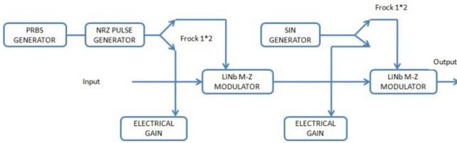
Fig. 1(a) Schematic diagram of CSRZ modulation format
