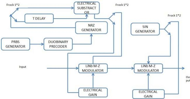
Fig. 3(a) Schematic diagram of CSRZ modulation format
