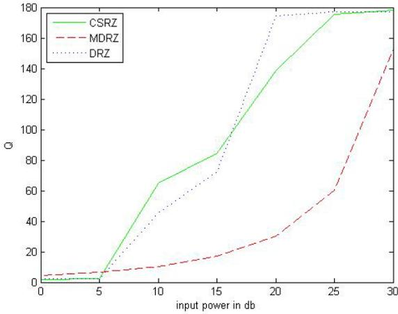
Fig.8 (a) Comparison of Q-Factors of modulations at 10Gbps
