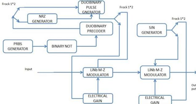
Fig. 2(a) Schematic diagram of DRZ modulation format
