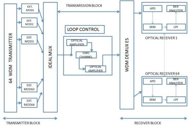
Fig. 4 Block diagram of the proposed system without Square Root Module
