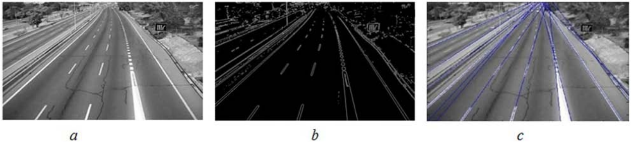
Figure 2. Intermediate results of detection of road region: (a) Background obtained through GMM (b)Result of Canny edge detector (c) Straight lines obtained using Standard Hough Transform
