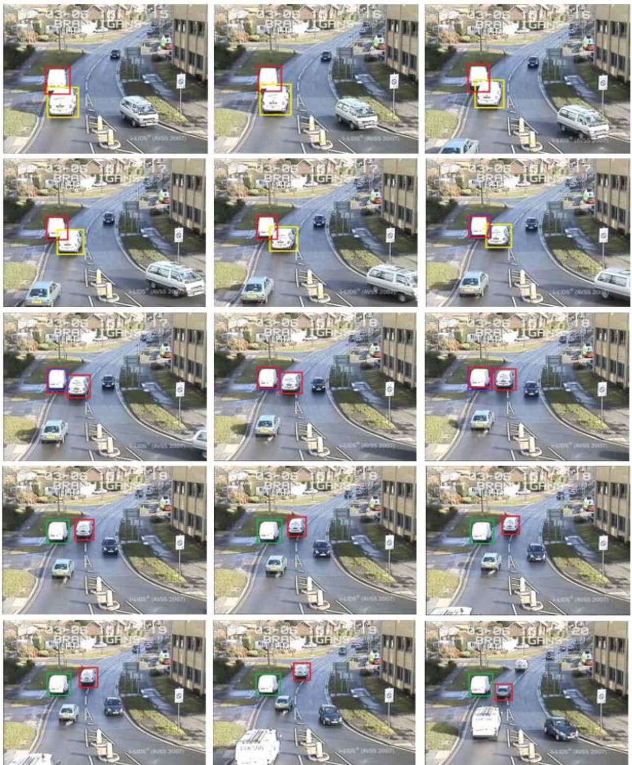
Figure 4. Visual results of our approach for vehicle abnormality detection and tracking, yellow color tracking window for near pass, red color tracking window for illegal lane crossing, green color tracking window for longtime stopped, and blue color tracking window for slow moving vehicle for AVSS PV Easy video sequence of i-Lids subset
