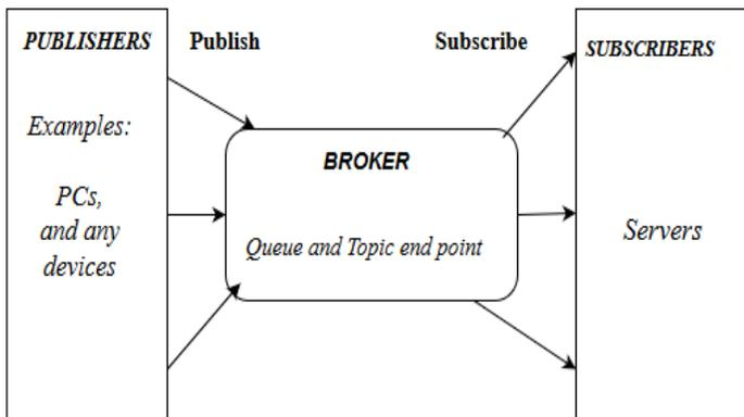
Figure 2: MQTT Architecture
