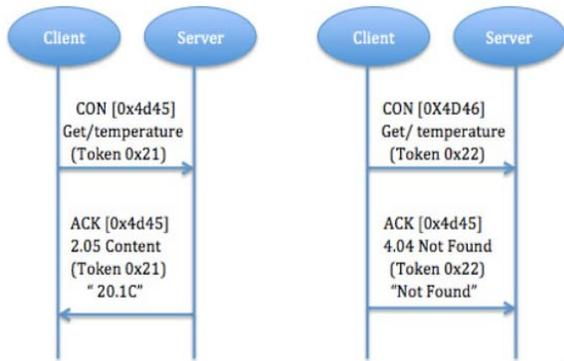
Figure 4: In piggy-backed, successful and failure response results of GET method [3].
