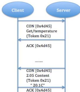
Figure 5: A Get request with a separate response [3].
