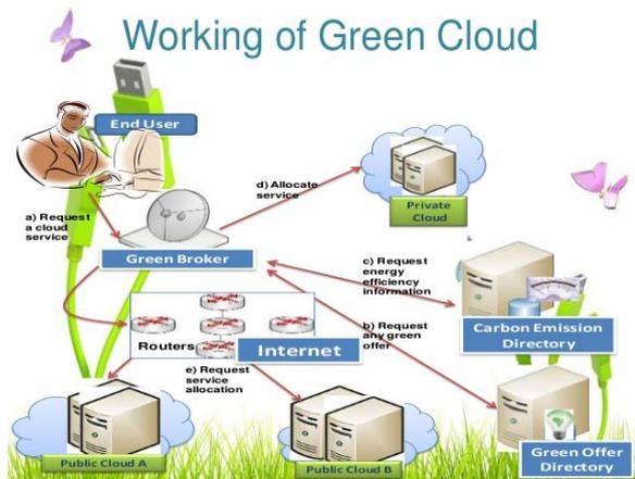
Figure 1. Working of Green Cloud Computing [2]
