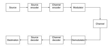
Fig. 3 Functional Block model of Communication System
