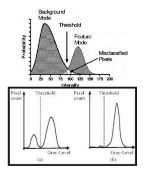
Figure 2. Histogram calculation image of thresholding
