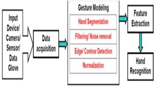
Figure 1. Generalized System Architecture for Hand Gesture Recognition
