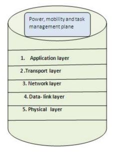
Fig.4. Protocol stack of sensor network
