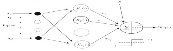
Fig. 4: Architecture of the SVM (N<sub>s</sub> is the number of support vectors).
