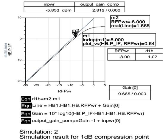
Figure.7 (a) Simulation for linearity.
