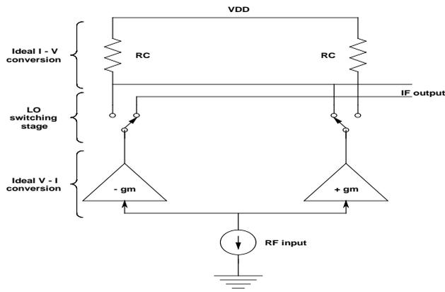
Figure. 2 illustrating diagram of Gilbert mixer cell
