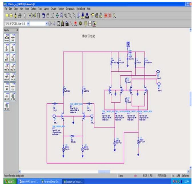
Figure.5 Simulated circuit of Current Folded mixer.
