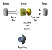
**Informatica Server**: TheInformatica Server extracts the source data, performs the data transformation, and loads the transformed data into the targets.
