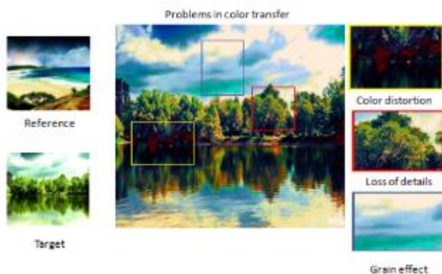
Fig. 1. Example-based color transfer [7] is an intuitional image manipulation technique, but it would produce some unexpected artifacts due to the complexity of color mapping. Grain effect, color distortion and loss of details appear in the transferred result commonly.
